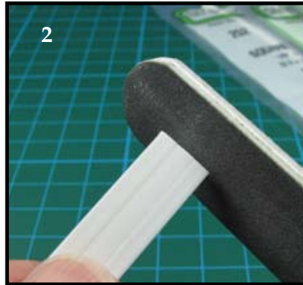
2. Glue the three lengths of Square Tube together to make a solid shape and use a sanding stick to make the ends flat and square.
